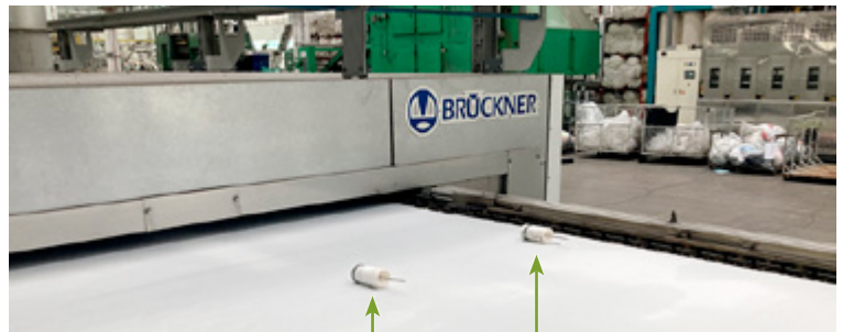
Measuring heads for dynamic determination of process temperatures
